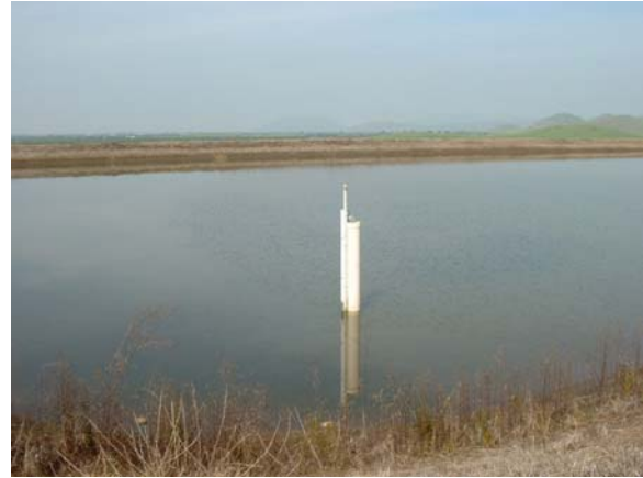
Water level monitoring and control devices in an OCID reservoir. There is a staff gauge on the left and a float device set in the PVC pipe on the right. The float device is connected to the telemetry system so that the water level can be monitored and controlled remotely or automatically.
