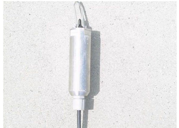
Figure 2. Telog PR-31 data collector.
