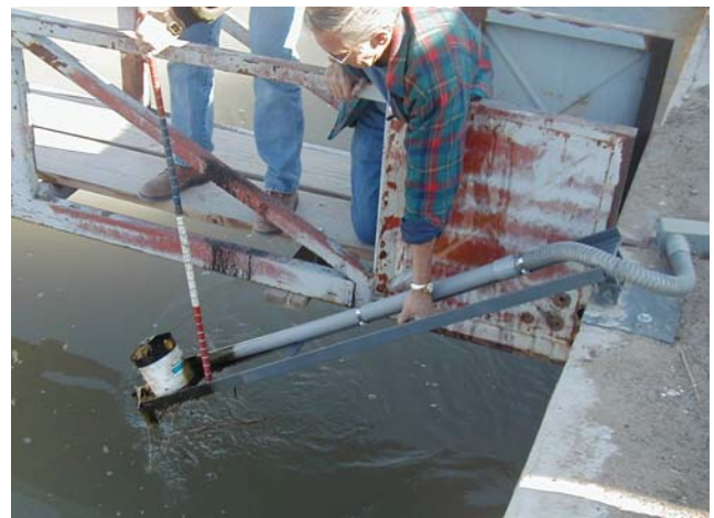
Figure 6. Mounting hardware for Argonaut SL at Truckee-Carson Irrigation District
