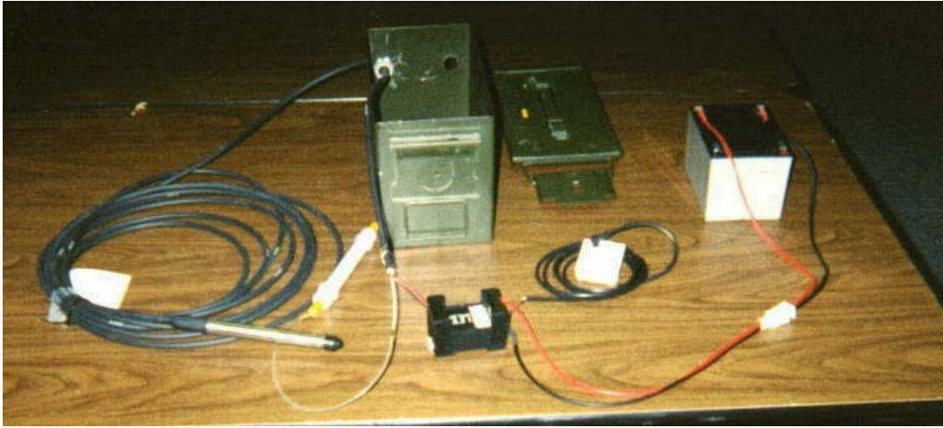
Photo 1. Components of portable water level monitoring package prior to installation in ammo box. This is the set up using the Druck pressure transducer and the ACR OWL datalogger.
