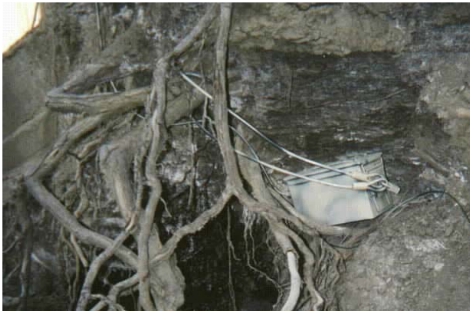
Photo 4. Ammo box with cable, lock, and paint.
