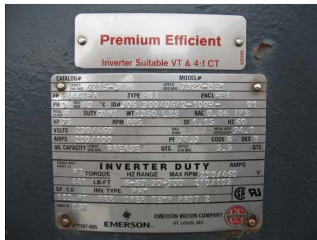
Example of inverter duty motor name plate
