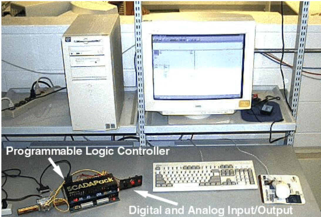
Figure 2. Automated System Hardware Setup
