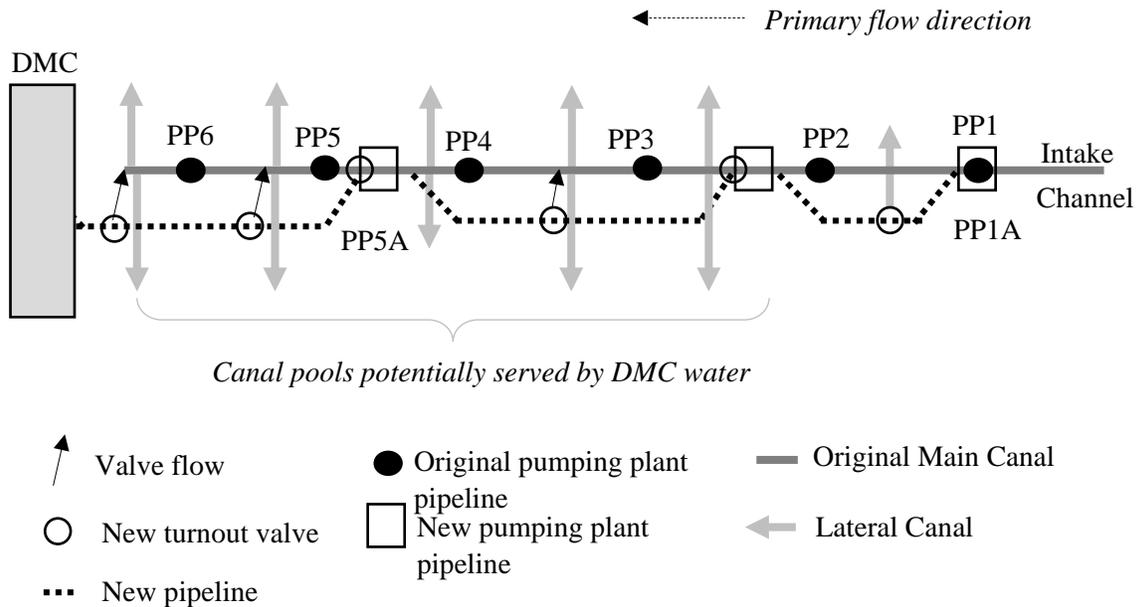
**Figure 3. Proposed Main Canal modernization plan. Two remote (manual) controlled sluice gates that operators can close at the DMC intertie are not shown.**
