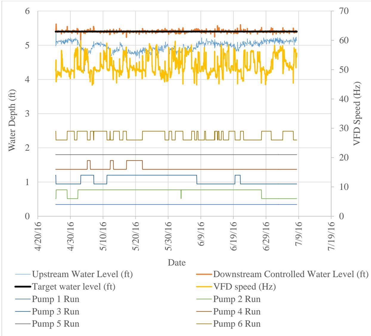
**Figure 2. Typical performance trending from Pumping Plant 4 under automatic downstream control, during peak irrigation season. Notice the VFD and single speed reactions required to maintain a relatively constant downstream water level. Individual pump capacities are roughly 40 CFS. Also, the “jumps” in *Pump Run* trends indicate pump starts/stops.**
