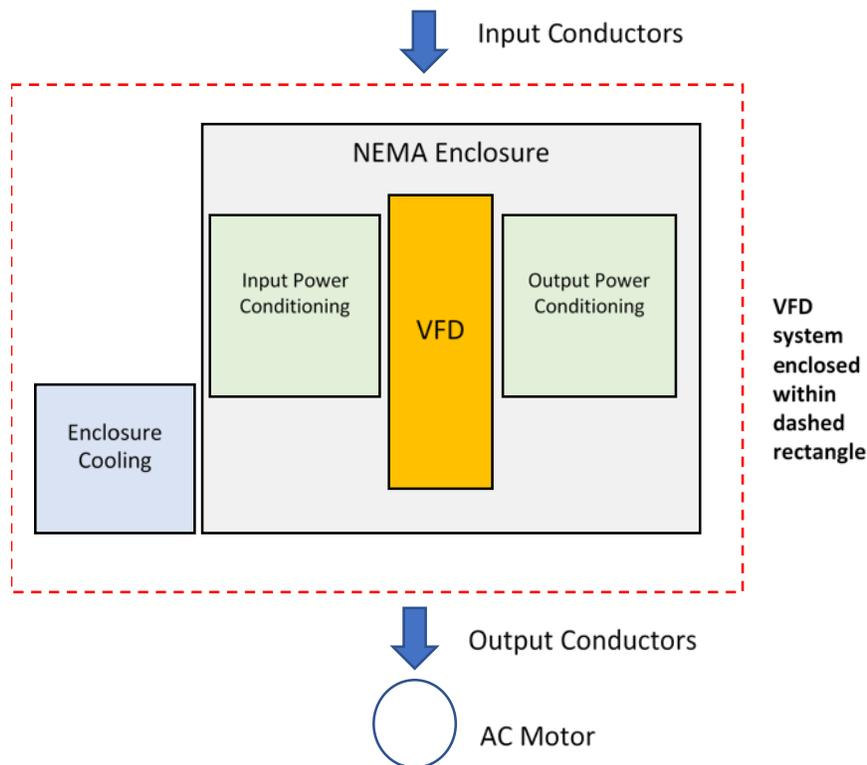
Figure 1. Major potential components of VFD systems
