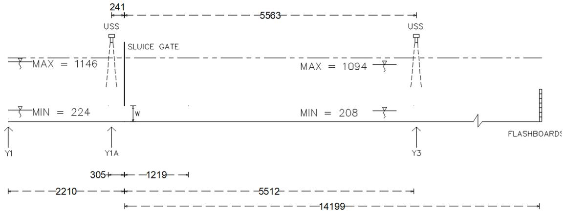
Fig. 2. Profile of test configuration. Units are mm.
