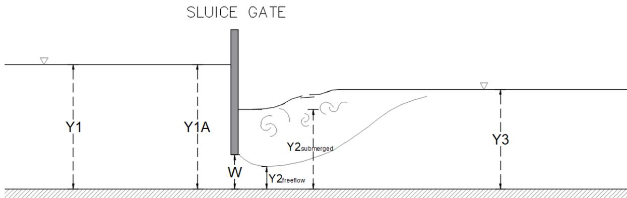
Fig. 1. Profile view of a sluice gate – horizontal floor
