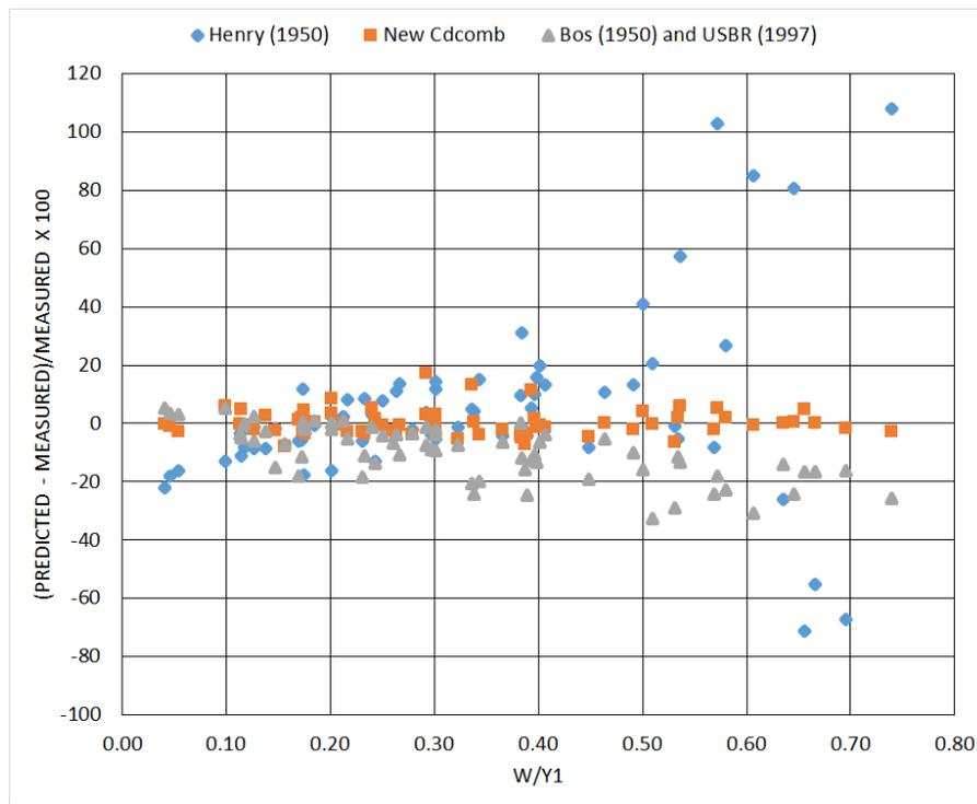
**Fig. 3.** Comparison of predicted versus measured submerged sluice gate flows using three techniques for estimating a discharge coefficient
