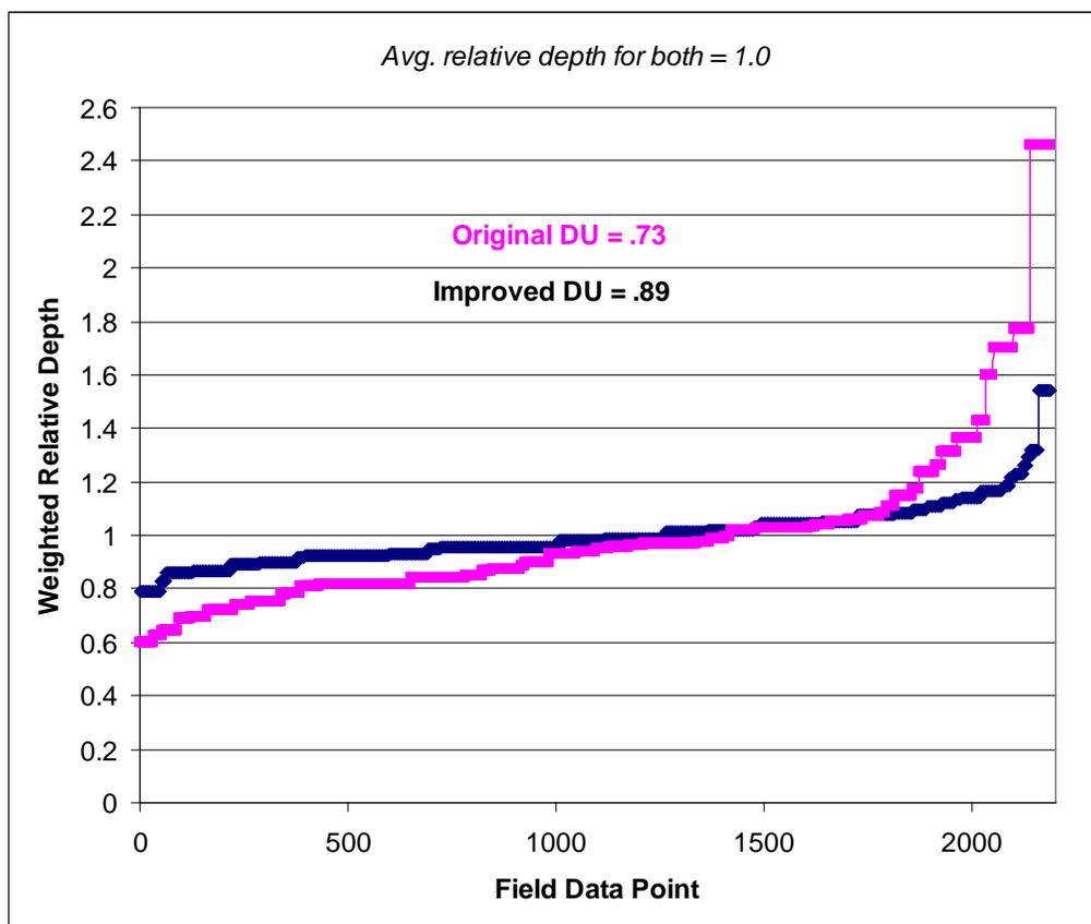
**Figure 3. 2007 catch can data for one of many project pivots, before and after improvements**
