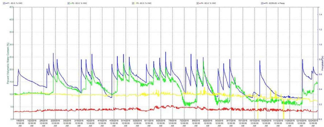
**Figure 1. Reasonable soil moisture sensor readings and trends representing irrigation events and depths. Sensor depths range from 2 feet to 10 feet.**
