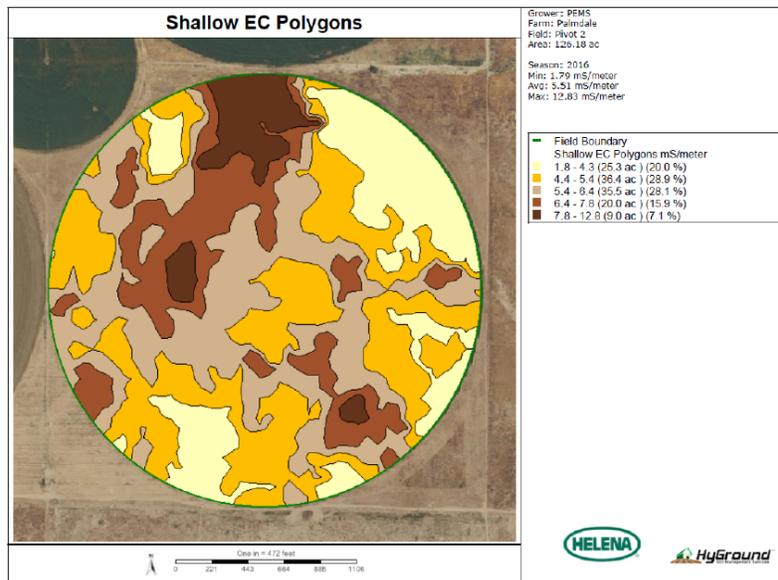
**Figure 8. Soil electroconductivity mapping example for one pivot; units in mS/meter**
