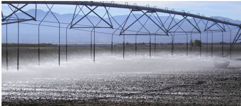
Figure 14. Drops strung over truss rods to increase the wetted area
