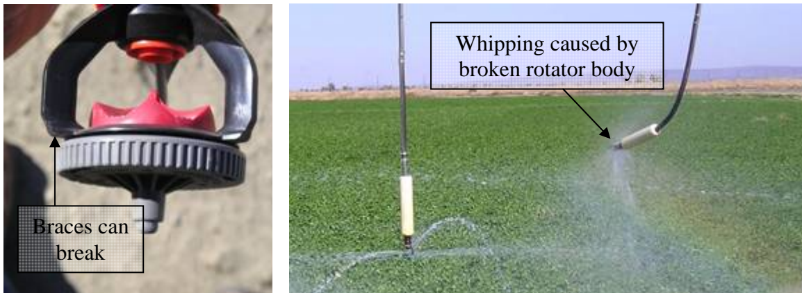
Figure 10. Non-functioning sprinkler because of broken rotator body
