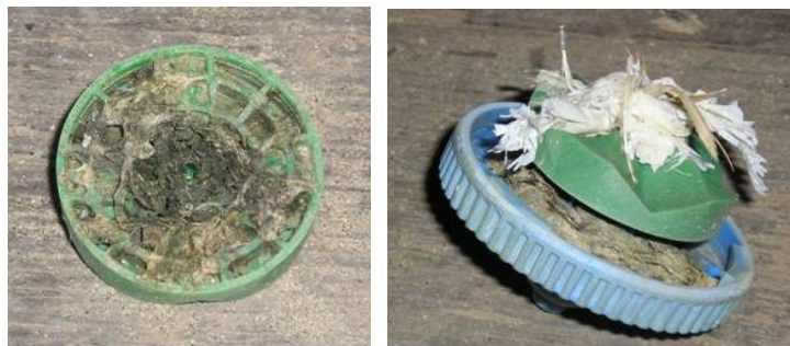
Figure 8. Sprinklers with trash on rotator plates
