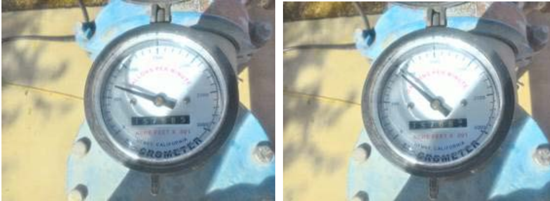
Figure 3. Participant 4's flow meter reading fluctuated continuously from low (left) to high (right) values as the photos were being taken
