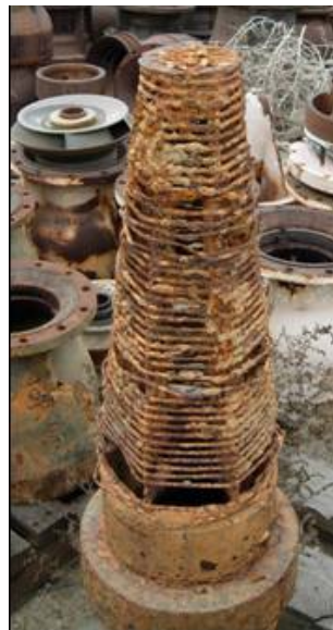
Figure 7. Corroded pump cone screen with missing sections.
