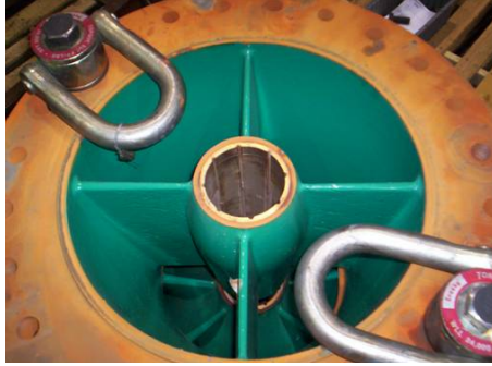
Figure 3. SK134 fusion bonded epoxy application.
