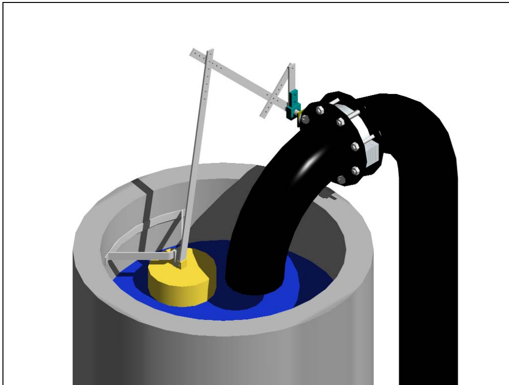
Figure 3. Present Design of an Up-and-Over Pressure Regulator for DEID.
